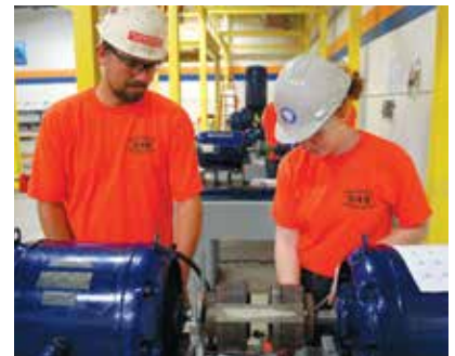
Millwrights Local 548 apprentices Michael Luger and Lisa Roragen demonstrate laser coupling alignment.
